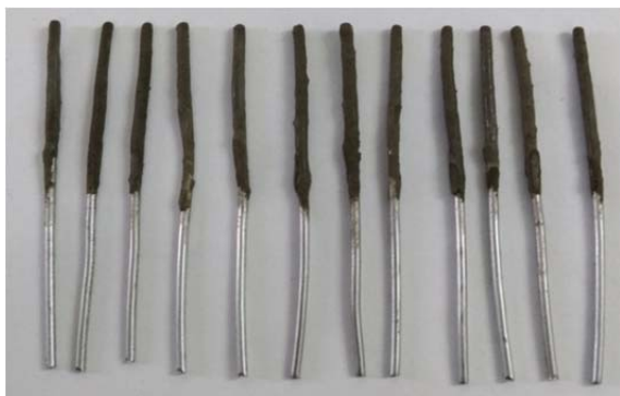
Fig. 1: Coated steel specimens
